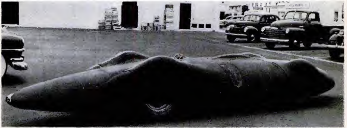
Side view of the Post-Hartelt hot rod displays its extreme streamlining. "Patch" on side is fuel tank
